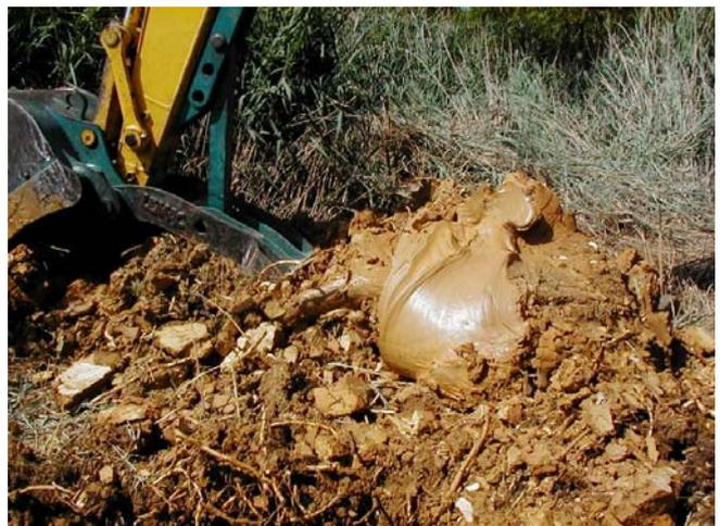
Figure 6. Hard, desiccated and soft, wet clayey washings at Test Pit 4
