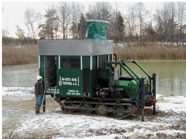
Figure 8. Track-mounted DMT rig.
