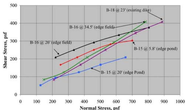
Figure 13. In-place drained shear strength of washings determined by borehole shear test.
