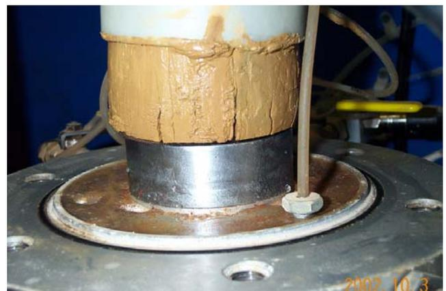
Figure 7. Sample of clayey washings expanding due to lack of confinement during extrusion from Shelby Tube.
