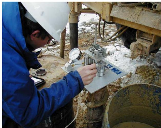
Figure 12. View of borehole shear head being raised.
