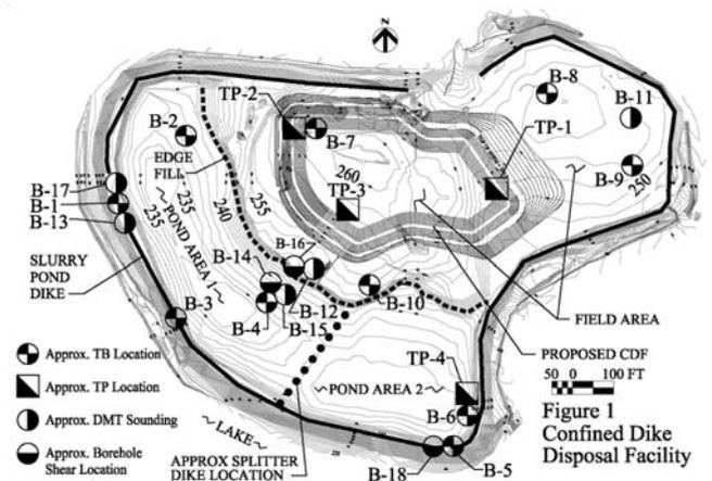
Figure 1. Confined Dike Disposal Facility
