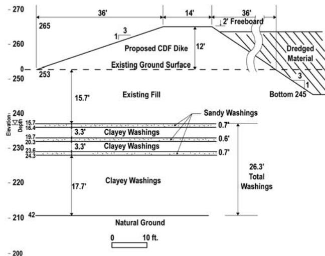
Figure 3. Typical CDF Section at Dilatometer Sounding B-12
